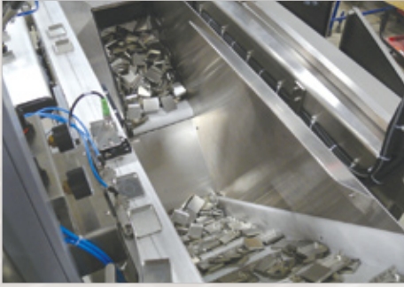
1. Bulk product and elevating conveyor
